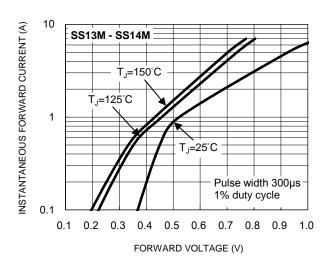
Fig.6 Typical Forward Characteristics
