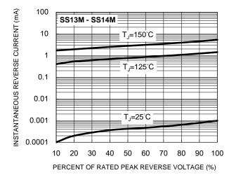
Fig.5 Typical Reverse Characteristics
